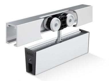
Sliding door fitting system for glass doors with a leaf weight of 140 kg and fixed panel and a 45 mm glass clamping plate attached to the ceiling
